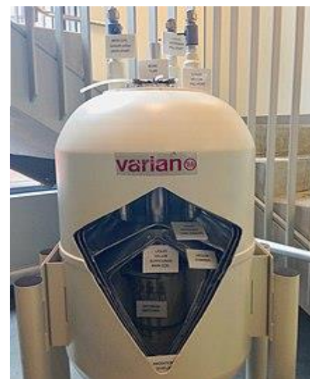
Cutaway of an NMR magnet that shows its structure: radiation shield, vacuum chamber, liquid nitrogen vessel, liquid helium vessel, and cryogenic shims.
